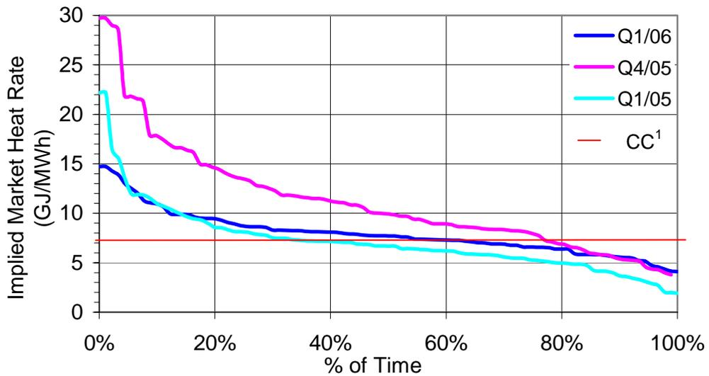
1 - CC denotes a representative combined-cycle generator with a heat rate of 7.5 GJ/MWh
