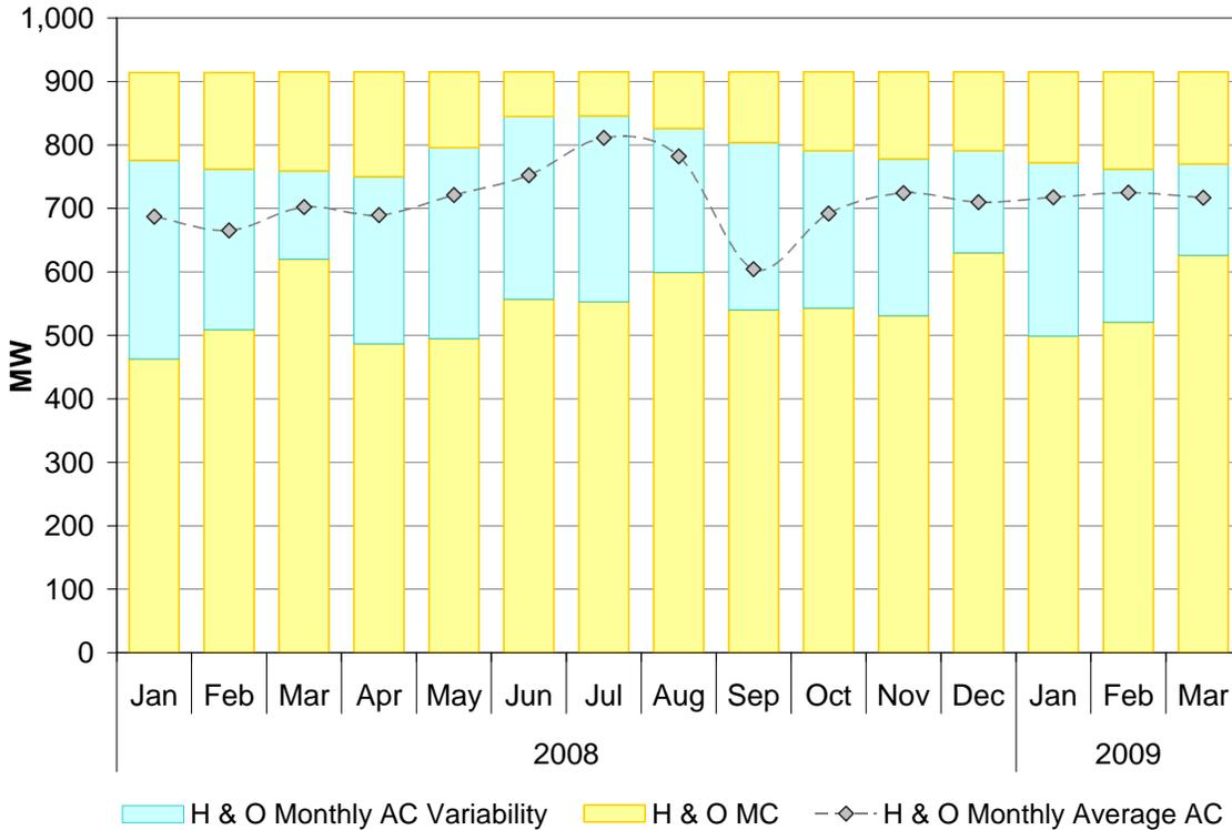
The MC is stable over the period of interest, and the monthly average AC varies seasonally, reflecting water conditions. The significant drop in average AC in September-08 was the result of maintenance at Brazeau.
